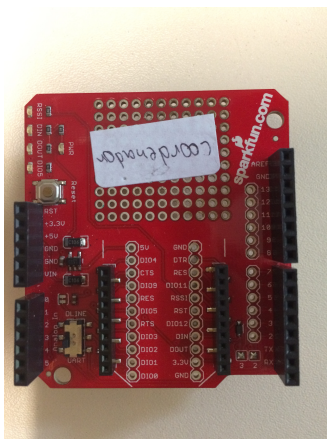
Figure 6. Expansion shield to connect XBee to Arduino Leonardo photograph.
