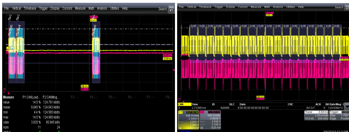
Figure 6 – a) Normal CAN bus 14% bus load; b) CAN bus under attack 100% bus load Source: from author
